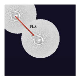
15. Set spot size to 0.2nm (Minimum size) and camera length to 60cm or 80cm. Insert a CL aperture 100um (#2) or 40nm (#3). Turn **SHIFT X** wobbler on. Stop wobbling using **Shift** and **Angle**. Follow above with **SHIFT Y**.
